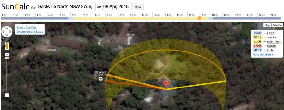
A sun arc allows us to see the path of the sun all year round. The area shown in Yellow is the arc of the sun with the upper limit being the winter arc and the lower limit summer.
